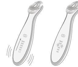
After two minutes, the light bars will glow on and off to indicate the current battery level. Once the device is fully charged, the lights will stop glowing on and off and the LED light bars will remain dimly lit.
