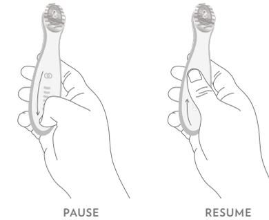
**TO STOP APPLICATION MANUALLY** During usage, you can stop the device at any time by swiping down the full length of the touch surface two times.
