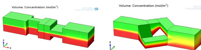
**Figure 1. COMSOL Multiphysics Modeling.** An example of a 2-stage turbulent mixer is shown on the left, and an example of a simple single-stage laminar mixer is shown on the right.
